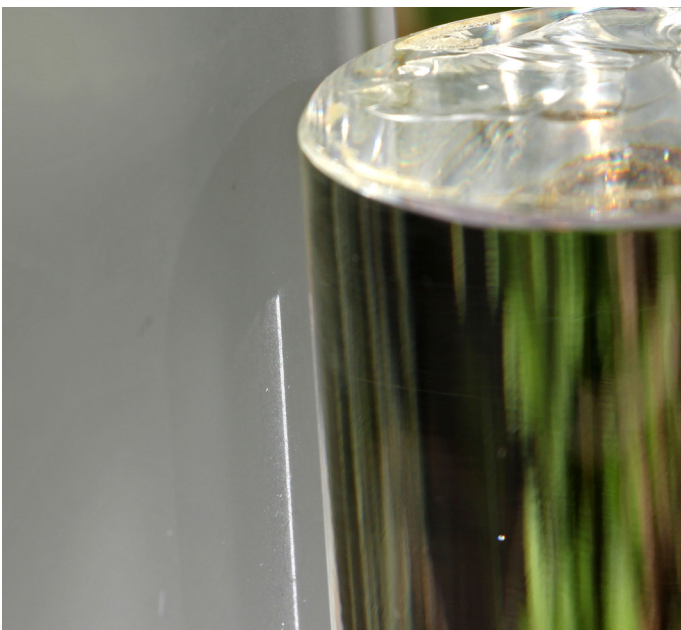
Fig. 10: The projection of a fine line of light onto etched glass
