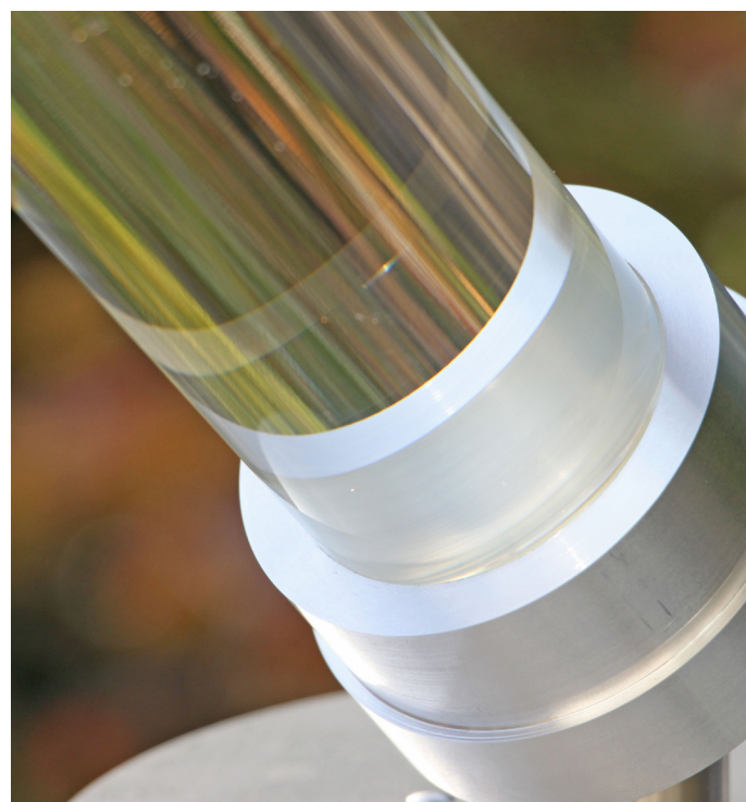
Fig. 3: Inside the glass tube is the cylindrical lens (D=50mm).
