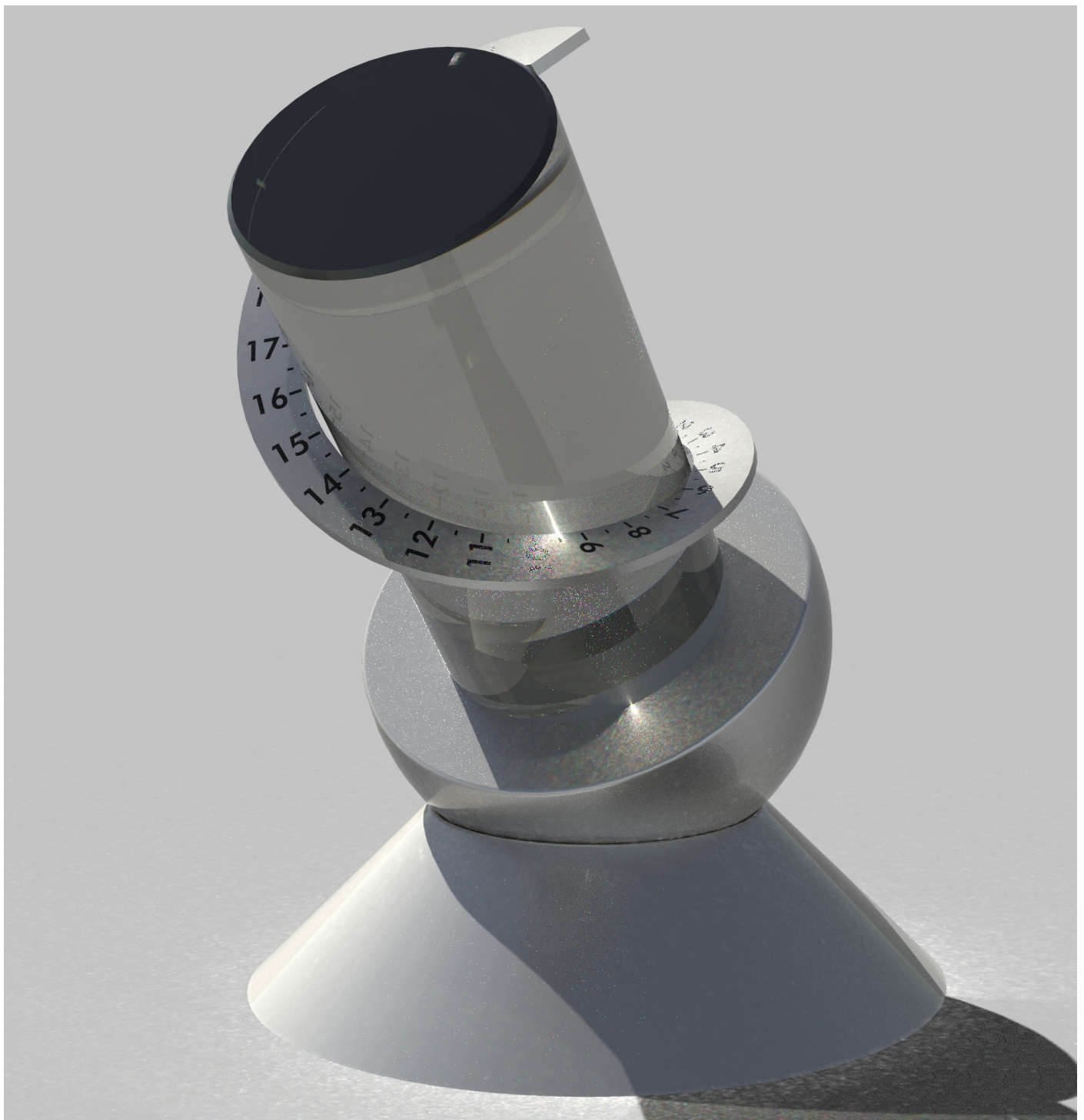
Fig. 20: The glass sundial at the summer solstice (20 th June) at 9:30 solar time (LAT) at latitude 50°N..
