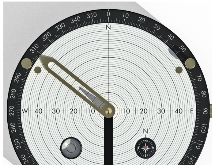
Figure 2: The direction of the shadow can be determined using the pointer placed on the gnomon. Here, it is 308.5^\circ from north.
