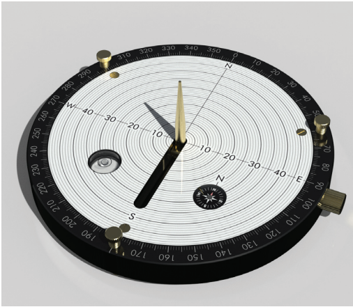
Figure 4a: The shadow length can be read on the circular scale and is currently 25 mm.
