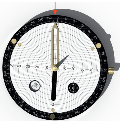
Figure 5c: The middle is at 357°. Mark the determined north direction there.
