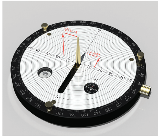
Figure 4b: At solar noon, the sun reaches its highest point. The shadow is at its shortest and measures 14 mm.
