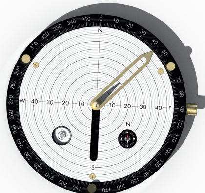
Figure 5b: In the afternoon, the shadow reaches the 20 mm circle again at 44°.
