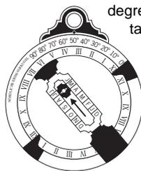
2. Adjust the runner on the date scale to the correct date by moving it up or down. On the back it will automatically show the corresponding declination of the sun, that is its angle to the celestial equator.
