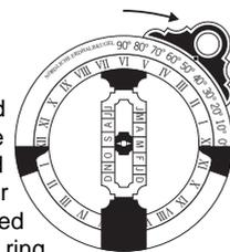
3. Open the hour ring until it touches the stoppers and stands exactly at a right angle to the meridian ring.
