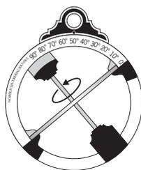
4. Hold the sundial by the cord in the suspension. Hold it to the sun and turn it slowly, until a ray of light comes through the hole in the cursor and falls into the centre of the inner rim of the hour ring. Here you can read Real Local Time. If necessary turn the face of the sun scale a little towards the sun.
